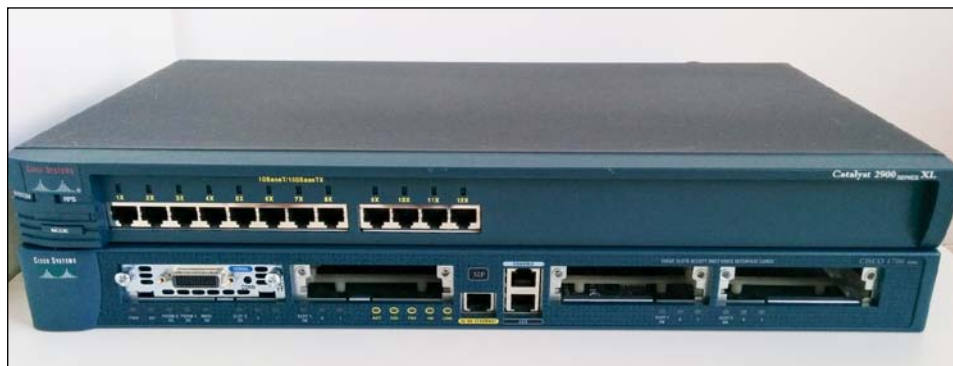
The Cisco switch and router
